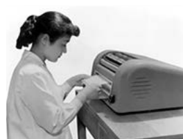
The Ricoh 101, Japan's first desktop diazo-wet copier to integrate exposure and development
