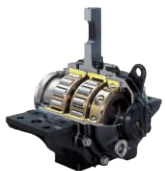
Cutaway of 0 Series Shinkansen axle bearings and housing
