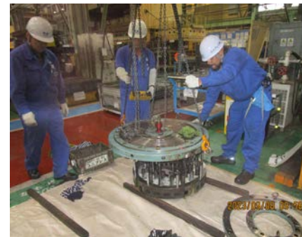
Intermediate press maintenance training (hands-on clutch/brake inspection training)
