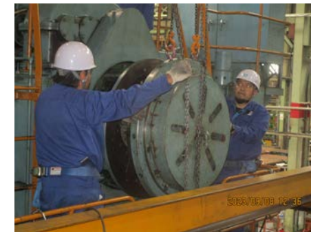
Intermediate press maintenance training (hands-on clutch/brake inspection training)
