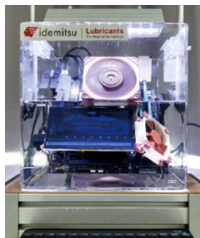
A test unit for the IDEMITSU ICF Series of immersion cooling oil for data centers. The series combines high safety with excellent cooling performance by drawing on the technological expertise we have cultivated in developing a wide range of lubricants. Contributing to energy savings at next-generation data centers
