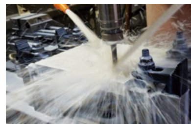
High-speed drilling of metal while spraying water-soluble cutting fluid diluted with water. The basic applications of cutting fluid include lubricating and cooling tools as well as preventing rust and cleaning machinery. Optimal formulation design of oil products contributes to higher productivity and a better working environment at processing sites.
