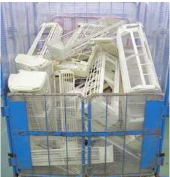
Polystyrene parts recovered from used air conditioners
