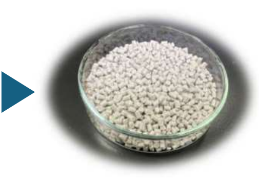
Material developed from recovered polystyrene
